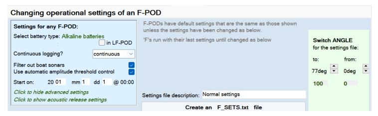
Select battery type: click the label to go through the options. This sets a minimum voltage for a stack of batteries, at which the POD will shift to the next stack on its list. The list starts with the weakest usable stack, so weak batteries are exhausted first in order to minimise discarding of part-used batteries.
