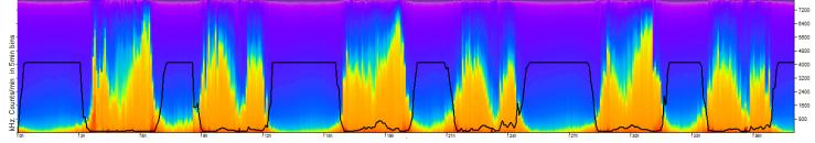
The noise display also shows vertical coloured bars. The colour represents the modal frequency (kHz) of the clicks logged. The height represents the Log of the sum of the squared sound pressure level (Pa) of logged clicks i.e. it accounts for the frequency response of the hydrophone.
