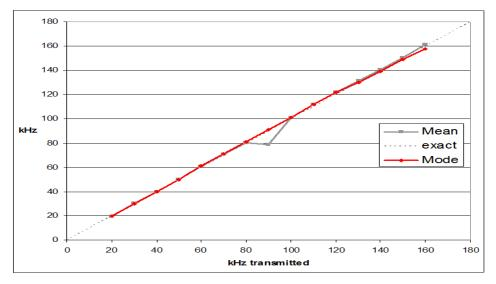
The frequency readout for pure tones of 10 cycles duration is shown above from tests by the National Physical Laboratory in the UK. At 90kHz some low values arise from an internal resonance.
