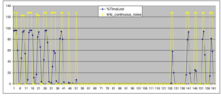
The sediment at this site generates noise at the mid to low end of the NBHF frequency range, and is so intense that many hours are maxing out – reaching the 4096 clicks limit in many minutes except during the neap phase of the tidal cycle.
