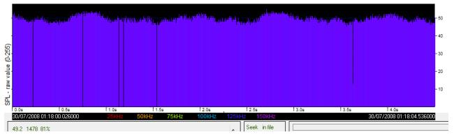
These data come from a rotational test of a POD. The mean SPL is 49.2, and the minimum is 81% of the maximum. 1478 clicks were used in the calculation.
