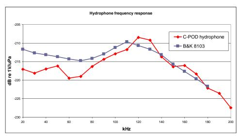
The frequency response (from tests by the National Physical Laboratory in the UK) of the C-POD hydrophone is shown above in comparison with the widely used B&K 8103.
