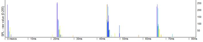
In the CP1 file the clicks arrived as multipath-replicates, that show variation in frequency (colour-coded in Sound Pressure Level displays), and great variation in SPL (height). These multi-path replicates are seen in many cetacean and boat sonar click trains and arise from sound reflections (echoes), and possibly from sound refraction as well.
