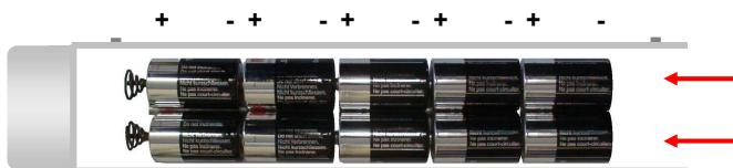
4. Fit the battery pack connector spring as shown below by squeezing the spring gently and passing the loop in the bottom of the spring over the rod. Then slide the spring down the rod until it touches the batteries.
