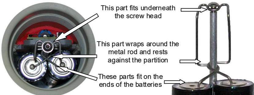
5. Adjust the screw in the top of the rod so that the dome of the screw is just below the top of the connector. This means you will only have to push the connector down approximately 7 mm to engage the head of the screw. This ensures that the battery pack is held securely, but not too tightly, as too much pressure could deform or damage the battery casings.
