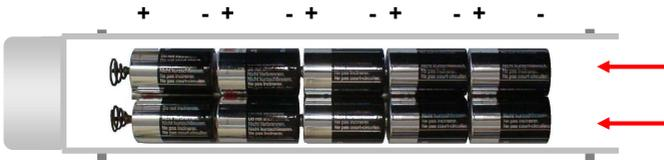
4. Fit the battery pack connector spring as shown below by squeezing the spring gently and passing the loop in the bottom of the spring over the rod. Then slide the spring down the rod until it touches the batteries.
