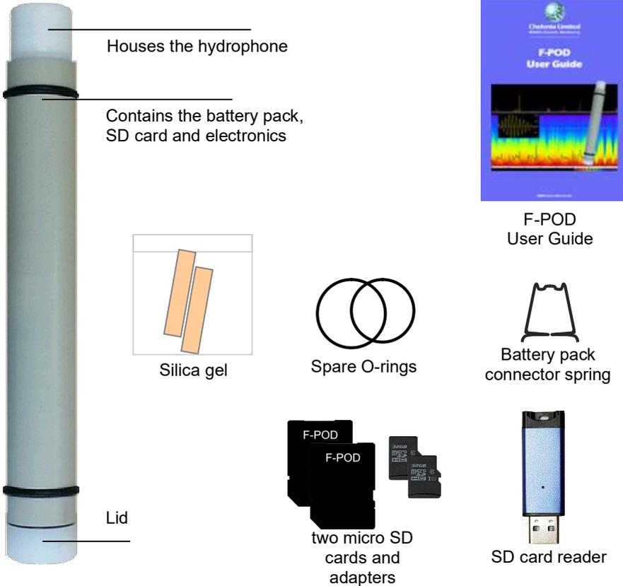
The F-POD consists of a polypropylene casing with hydrophone housing at one end and a removable lid at the other end.
