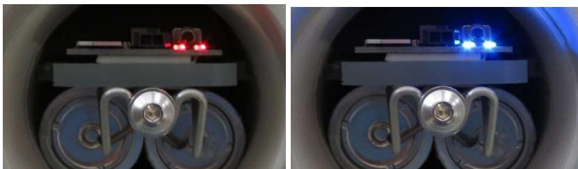
Both LEDs light red while the POD starts up, then blue to indicate that both battery stacks are OK (FPODs 6800 onwards will also light both LEDs white for a few seconds, then usually a single blue flash). Finally both LEDs flash green 5 times to indicate that the POD has started running.
