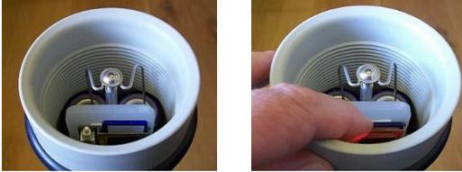
The POD electronics checks that each battery stack is providing power. The LED should give two short flashes per second, to indicate that both battery stacks are OK. If the LED gives a single flash, one of the battery stacks is faulty.
