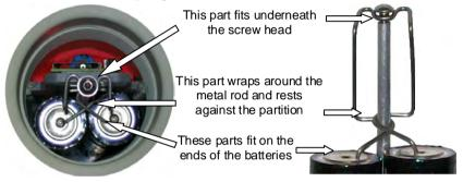
6. Adjust the screw in the top of the rod so that the dome of the screw is just below the top of the connector. This means you will only have to push the connector down approximately 7 mm to engage the head of the screw. This ensures that the battery pack is held securely, but not too tightly, as too much pressure could deform or damage the battery casings.
