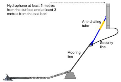
Design the mooring using a mixture of sinking ropes and buoyant ropes. Use sinking ropes so that no loops of cordage float at the surface to entangle propellers and buoyant ropes that do not lie on the bottom and suffer excessive abrasion.
