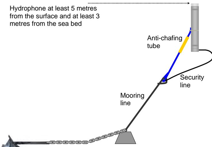
Design the mooring using a mixture of sinking ropes and buoyant ropes. Use sinking ropes so that no loops of cordage float at the surface to entangle propellers and buoyant ropes that do not lie on the bottom and suffer excessive abrasion.
