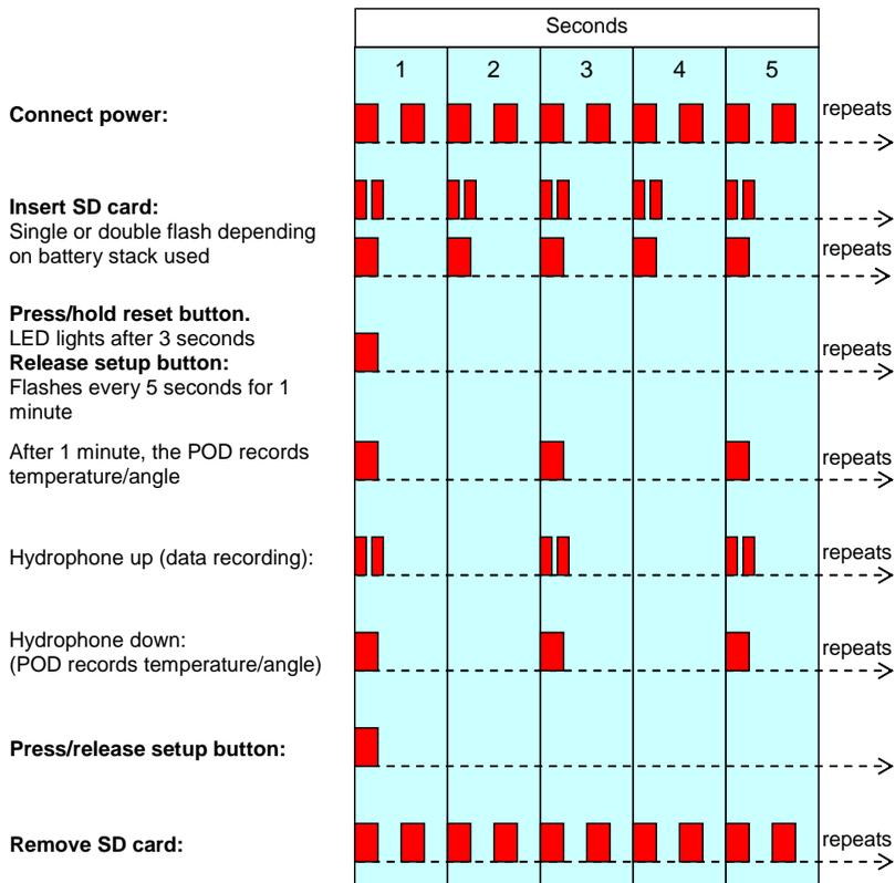
*When I opened the C-POD after deployment, the power LED was off.*
